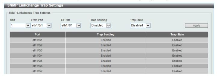
Figure 4-9SNMP Linkchange Trap Settings Window
