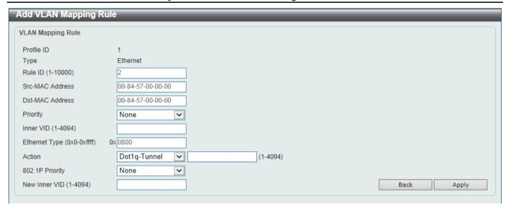
Figure 5-49VLAN Mapping Profile (Ethernet, Add Rule) Window
