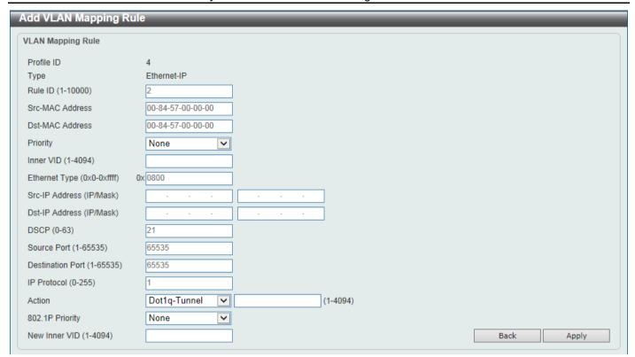
Figure 5-52VLAN Mapping Profile (Ethernet-IP, Add Rule) Window
