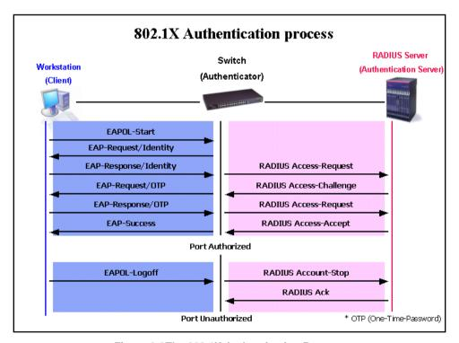
Figure 9-9The 802.1X Authentication Process
