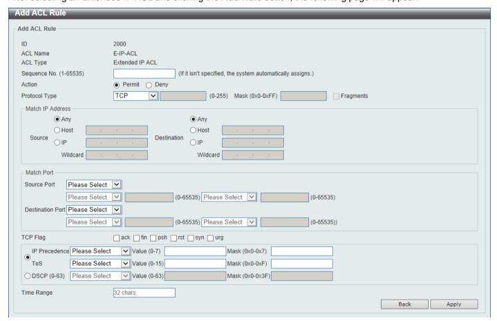
Figure 8-12Extended IP ACL (Add Rule) Window
