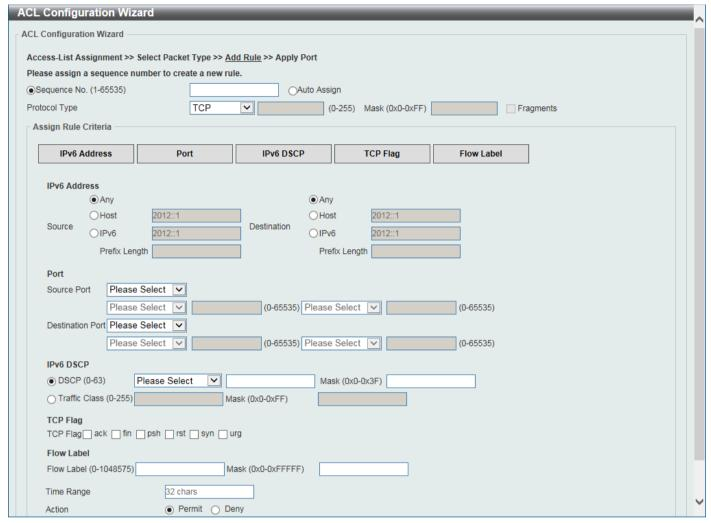
Figure 8-6ACL Configuration Wizard (Create, Packet Type, IPv6) Window
