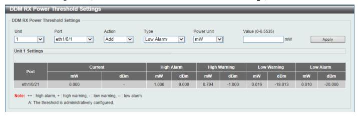
Figure 10-32DDM RX Power Threshold Settings Window
