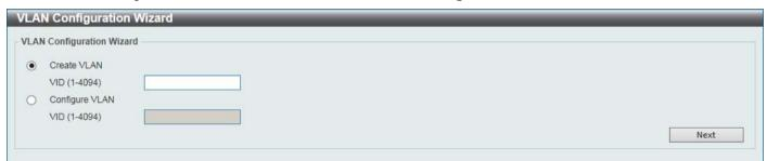
Figure 5-9 VLAN Configuration Wizard(Select VLAN) Window
