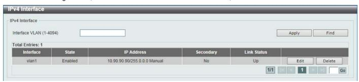
Figure 6-7IPv4 Interface Window
