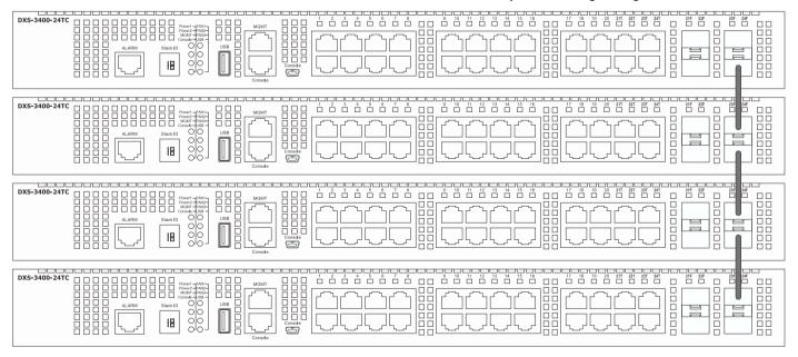
Figure 4-77Duplex Chain stacking topology (SFP+)
