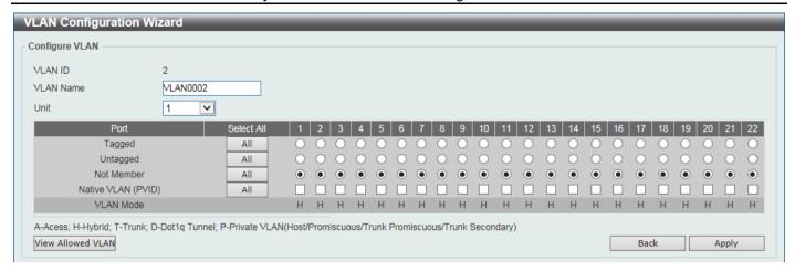
Figure 5-11VLAN Configuration Wizard (Configure VLAN) Window
