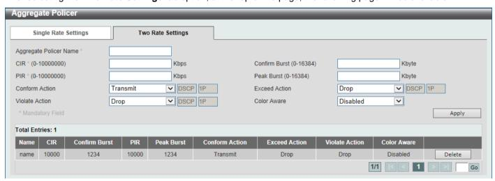
Figure 7-15Aggregate Policer (Two Rate Settings) Window
