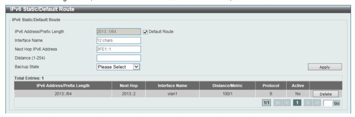
Figure 6-23IPv6 Static/Default Route Window
