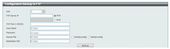
Figure 13-16Configuration Backup to FTP Window
