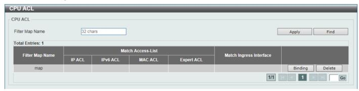
Figure 8-23CPU ACL Window
