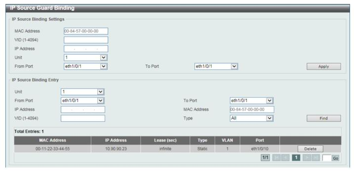
Figure 9-52IP Source Guard Binding Window
