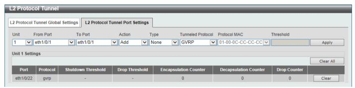
Figure 5-74L2 Protocol Tunnel (L2 Protocol Tunnel Port Setting) Window
