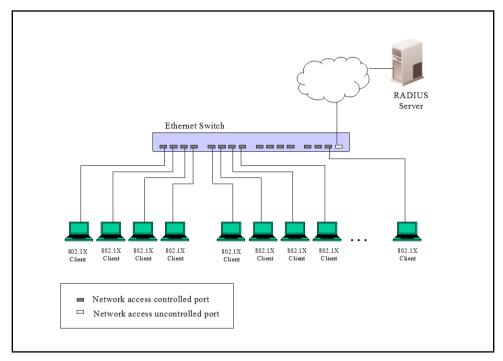
Figure 9-10Example of Typical Port-based Configuration
