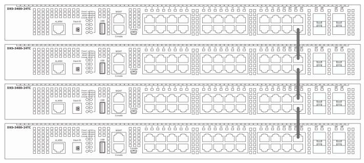
Figure 4-76Duplex Chain stacking topology (RJ45)
