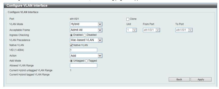
Figure 5-17VLAN Interface (Hybrid) Window
