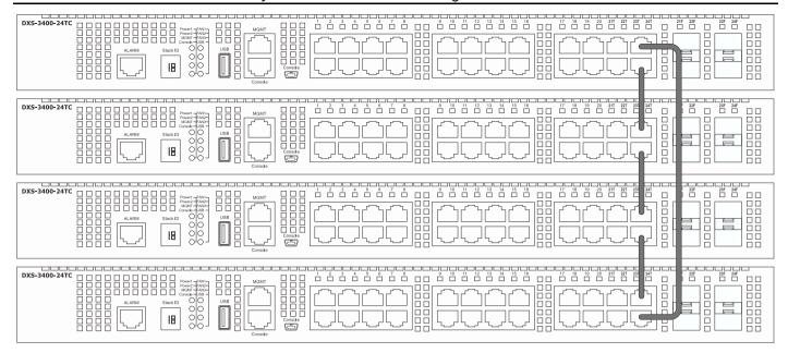
Figure 4-78Duplex Ring stacking topology (RJ45)
