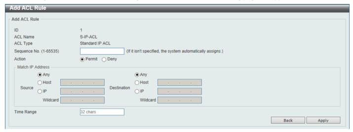
Figure 8-11Standard IP ACL (Add Rule) Window
