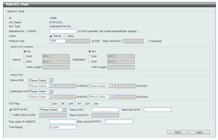
Figure 8-14Extended IPv6 ACL (Add Rule) Window
