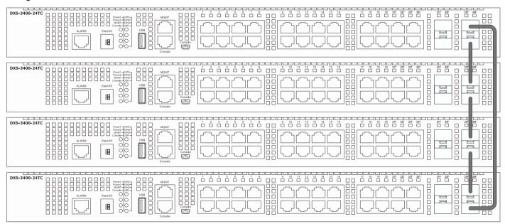
Figure 4-79Duplex Ring stacking topology (SFP+)
