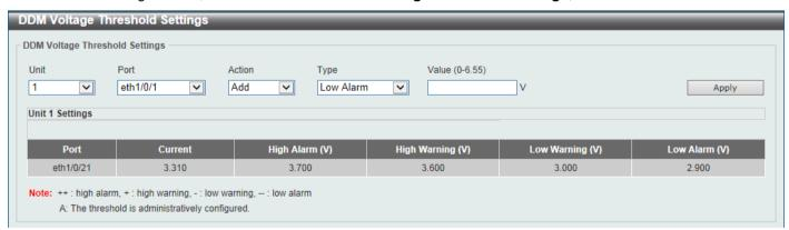
Figure 10-29DDM Voltage Threshold Settings Window
