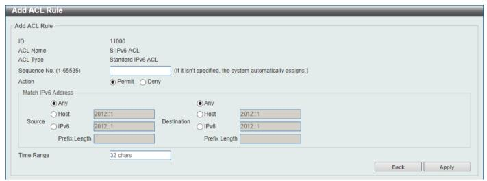
Figure 8-13Standard IPv6 ACL (Add Rule) Window
