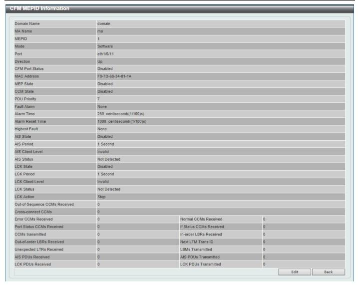
Figure 10-6CFM Settings (Add MA, Add MEP, MEPID Detail) Window
