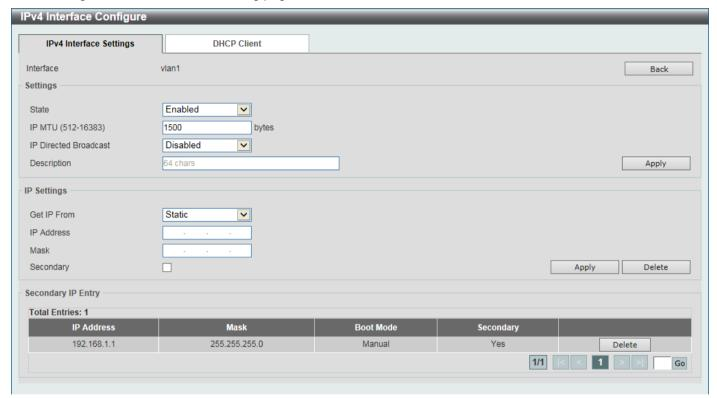
Figure 6-8IPv4 Interface (Edit) Window
